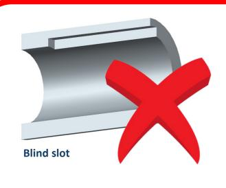
DO NOT ATTEMPT TO MACHINE A BLIND SLOT ie, A SLOT WITHOUT ANY TOOL RUNOUT
